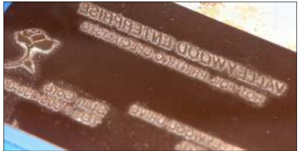
Image Number 2: Polymer Hot Foil Plate
