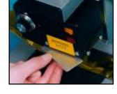
Slide the type holder or die holding block into the machine and you are almost ready to print!
